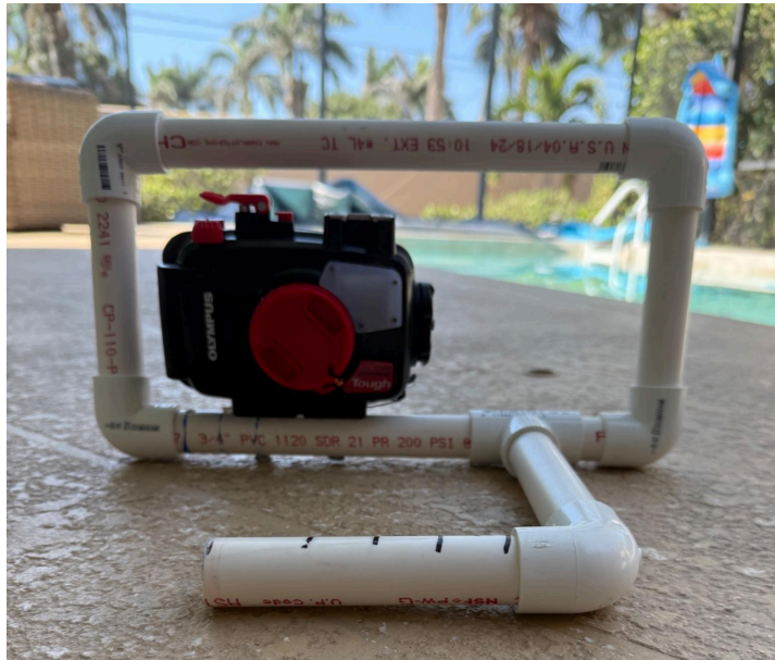
Figure 1. Custom PVC frame for capturing standardized photos. The arm outstretched away from the camera frame has sharpie marks indicating every half inch to calibrate the images so accurate distances were measured.
