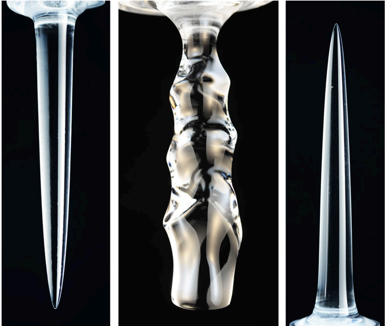
Fig. 5-1. The temperature of the water bath determines the shape of a melting cylinder of ice: 4 °C (left), 5.6 °C (center), and 8 °C (right). Photos courtesy of Department of Physics, New York University, New York, New York 10003, USA.
